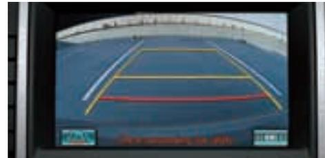
Back guide monitor (Optional): It supports smooth reversing operations when parking in a garage or parallel parking, showing the rear view taken by a camera integrated into the rear of the vehicle, together with guidelines on the display.
