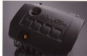
DUAL VVT-i 1.8-liter/Gasoline/Unleaded/2ZR-FE 134HP/6000rpm (SAE net) 17.8kg-m/4400rpm (SAE net)
